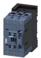
power contactor, AC-3e/AC-3, 95 A, 45 kW / 400 V, 3-pole, 230 V AC, 50 Hz, auxiliary contacts: 1 NO + 1 NC, main circuit: screw terminal, control and auxiliary circuit: spring-loaded terminal, size: S3
