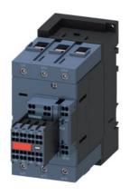
power contactor, AC-3e/AC-3, 95 A, 45 kW / 400 V, 3-pole, 24 V DC, 0.8-1.2\* Us, with integrated varistor, auxiliary contacts: 1 NO + 1 NC, integrated varistor, main circuit: screw terminal, control and auxiliary circuit: spring-loaded terminal, size: S3, suitable for PLC outputs, captive auxiliary switch
