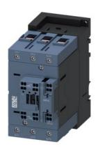
power contactor, AC-3e/AC-3, 95 A, 45 kW / 400 V, 3-pole, 20-33 V AC/DC, 50/60 Hz, with integrated varistor, auxiliary contacts: 1 NO + 1 NC, main circuit: screw terminal, control and auxiliary circuit: spring-loaded terminal, size: S3, communication-capable
