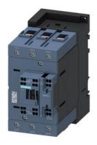
power contactor, AC-3e/AC-3, 95 A, 45 kW / 400 V, 3-pole, 175-280 V AC/DC, 50/60 Hz, with integrated varistor, auxiliary contacts: 1 NO + 1 NC, main circuit: screw terminal, control and auxiliary circuit: spring-loaded terminal, size: S3  $\,$
