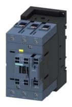
power contactor, AC-3e/AC-3, 95 A, 45 kW / 400 V, 3-pole, 175-280 V AC/DC, 50/60 Hz, with integrated varistor, auxiliary contacts: 1 NC, main circuit: screw terminal, control and auxiliary circuit: spring-loaded terminal, size: S3, F-PLC-IN
