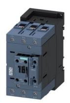
power contactor, AC-3e/AC-3, 110 A, 55 kW / 400 V, 3-pole, 24 V AC, 50 Hz, auxiliary contacts: 1 NO + 1 NC, screw terminal, size: S3, upright mounting position
