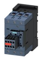
power contactor, AC-3e/AC-3, 110 A, 55 kW / 400 V, 3-pole, 110 V AC, 50 Hz / 120 V, 60 Hz, auxiliary contacts: 2 NO + 2 NC, screw terminal, size: S3, captive auxiliary switch
