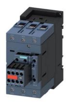
power contactor, AC-3e/AC-3, 110 A, 55 kW / 400 V, 3-pole, 230 V AC, 50/60 Hz, with plugged-in varistor, auxiliary contacts: 2 NO + 2 NC, screw terminal, size: S3, captive auxiliary switch
