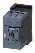
power contactor, AC-3e/AC-3, 110 A, 55 kW / 400 V, 3-pole, 20-33 V AC/DC, 50/60 Hz, with integrated varistor, auxiliary contacts: 1 NO + 1 NC, screw terminal, size: S3, communication-capable
