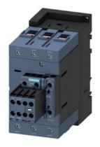
power contactor, AC-3e/AC-3, 110 A, 55 kW / 400 V, 3-pole, 20-33 V AC/DC, 50/60 Hz, with integrated varistor, auxiliary contacts: 2 NO + 2 NC, screw terminal, size: S3, removable auxiliary switch
