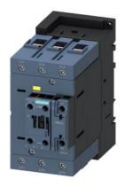
power contactor, AC-3e/AC-3, 110 A, 55 kW / 400 V, 3-pole, 175-280 V AC/DC, 50/60 Hz, with integrated varistor, auxiliary contacts: 1 NC, screw terminal, size: S3, F-PLC-IN
