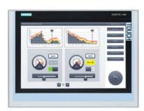
SIPLUS HMI TP1500 Comfort based on 6AV2124-0QC02-0AX1 with conformal coating, 0...+50 °C, Comfort Panel, touch operation, 15" widescreen TFT display, 16 million colors, PROFINET interface, MPI/PROFIBUS DP interface, 24 MB configuration memory, WEC 2013, configurable as of WinCC Comfort V14 SP1 with HSP
