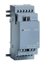
SIPLUS LOGO! DM8 24 based on 6ED1055-1CB00-0BA2 with conformal coating, -40...+70 °C, start up -25 °C, expansion module, power supply / I/O: 24 V/24 V/trans., 4 DI/4 DQ for LOGO! 8
