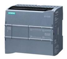
SIPLUS S7-1200 CPU 1214C DC/DC/relay based on 6ES7214-1HG40-0XB0 with conformal coating, -40...+70 °C, start up -25 °C, signal board: 0, compact CPU, DC/DC/relay, onboard I/O: 14 DI 24 V DC; 10 DQ relay 2 A 2 AI 0-10 V DC, power supply: DC 20.4-28.8 V DC, program/data memory 100 KB
