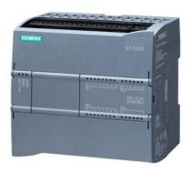
SIPLUS S7-1200 CPU 1214C DC/DC/relay based on 6ES7214-1HG40-0XB0 with conformal coating, -40...+60 °C, start up -25 °C, compact CPU, DC/DC/relay, onboard I/O: 14 DI 24 V DC; 10 DQ relay 2 A; 2 AI 0-10 V DC, power supply: AC 20.4-28.8 V DC, program/data memory 100 KB
