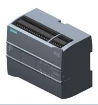
SIPLUS S7-1200 CPU 1215C AC/DC/relay based on 6ES7215-1BG40-0XB0 with conformal coating, -40...+60 °C, start up -25 °C, compact CPU, AC/DC/relay, 2 PROFINET ports onboard I/O: 14 DI 24 V DC; 10 DQ relay 2 A; 2 AI 0-10 V DC, 2 AQ 0-20 mA DC power supply: AC 85-264 V AC @ 47-63 Hz, program/data memory 125 KB
