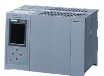
SIPLUS S7-1500 CPU 1517H-3 PN based on 6ES7517-3HP00-0AB0 with conformal coating, 0...+60 °C, central processing unit with 2 MB work memory for program and 8 MB for data, 1st interface: PROFINET IRT with 2-port switch, 2nd interface: PROFINET RT, 3rd interface: H-SYNC, SIMATIC Memory Card required
