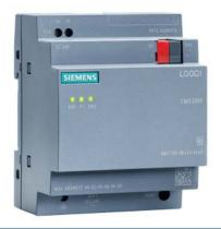
LOGO! CMK2000 Communication module for integrating the LOGO! 8 "in the building system bus KNX;" connection 24 V DC 0.04A 1 RJ45 port for Ethernet 50 communication objects time-of-day synchronization Configuration/diagnostics via web interface
