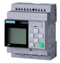
LOGO! 230RCE,logic module, display power supply / I/O: 115 V/230 V/relay, 8 DI/4 DO, memory 400 blocks, modularly expandable, Ethernet, integrated web server, data log, user-defined web pages, standard microSD card for LOGO! Soft Comfort V8.4 or higher, older projects executable cloud connection, MQTT in all LOGO! 8.4 basic units
