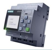
LOGO! 12/24RCE, logic module, display power supply / I/O: 12/ 24 V DC/relay, 8 DI (4 AI)/4 DO, memory 400 blocks, modularly expandable, Ethernet, integrated web server, data log, user-defined web pages, standard microSD card for LOGO! Soft Comfort V8.4 or higher, older projects executable cloud connection, MQTT in all LOGO! 8.4 basic units
