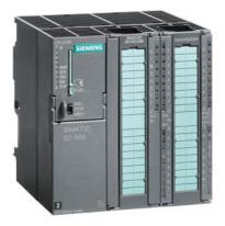
SIMATIC S7-300, CPU 313C, Compact CPU with MPI, 24 DI/16 DO, 4 AI, 2 AO, 1 Pt100, 3 high-speed counters (30 kHz), Integr. power supply 24 V DC, work memory 128 KB, Front connector (2x 40-pole) and Micro Memory Card required
