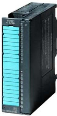
SIMATIC S7-300, Analog input SM 331, isolated, 2 AI, Resolution 9/12/14 bits, U/I/thermocouple/resistor, alarm, diagnostics, 1x 20-pole, Removing/inserting with active backplane bus
